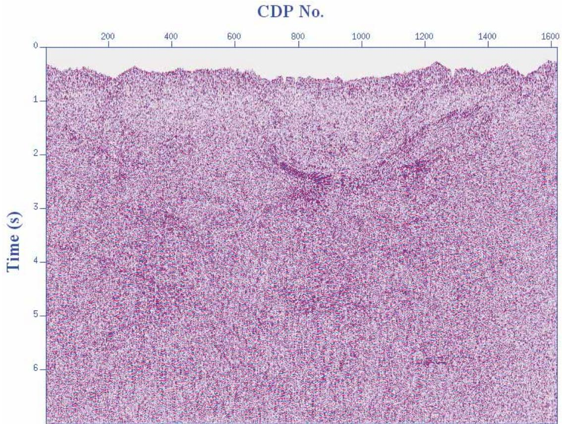
**Figure 2** The CMP-stacked section of the Izeh data. The S/N ratio of the section is low due to the complex structure. Many events are missing for the same reason.
