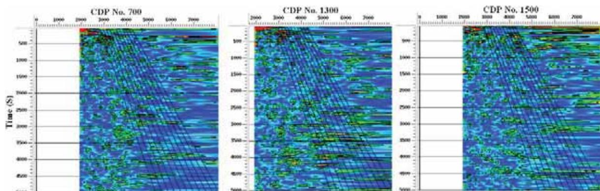
**Figure 1** The Velocity spectra for some CDPs that shows the difficulty of velocity picking for this complex structure.
