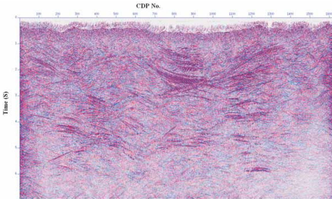
**Figure 3** The CRS-stacked section of the Izeh data. The S/N ratio of the section is significantly high and more events can be seen that completely show the folding.
