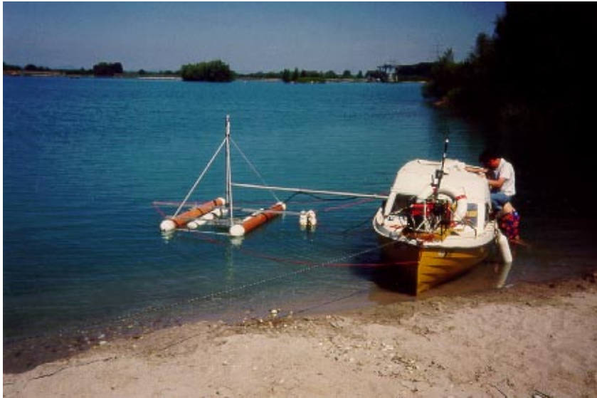
Figure 4.14: Field equipment: the sonic boomer is located on the left hand side of the derrick, the hydrophone in the middle. The power source and the computers are located aboard.
